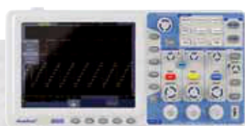
color digital oscilloscope 30 Mhz
